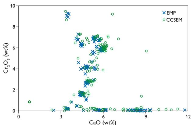
Fig. 3. Comparison of electron microprobe (EMP) and CCSEM measurements for chromium oxide and calcium oxide in Mg-rich garnets from diamond-bearing rocks. Note the good correlation between the results obtained with CCSEM and the EMP data.
