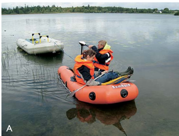
Fig. 3. A: Mapping of lake sediments using reflection ground penetrating radar (GPR). The radar equipment is contained in the grey rubber boat. B: An example of a GPR reflection profile with a preliminary interpretation.
