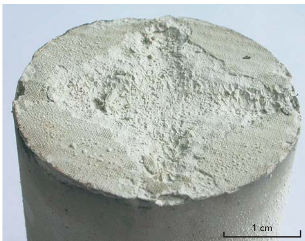
Fig. 5. The inlet end of the composite sample showed a dissolution structure after flooding with CO 2 -enriched water. The star-like shape is governed by the arrangement of the distributor channels in the end pieces of the core holder.
