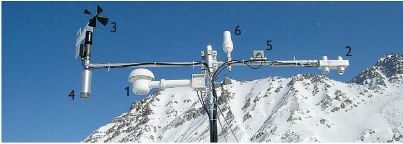
Fig. 2. The automatic weather station: 1 : aspirated radiation shield for air temperature and humidity probes. 2 : radiometers for shortwave and longwave incoming and outgoing radiation. 3 : sensor for wind speed and direction. 4 : sensor to measure snow surface level. 5 : two-axes tilt sensor of the instruments boom. 6 : Iridium satellite antenna. 7 : Iridium satellite radio. 8 : atmospheric pressure. 9 : sensor to measure ice-surface level. 10 : thermistor string for ice temperature (drilled into the ice). 11 : ablation sensor. 12 : GPS antenna.
