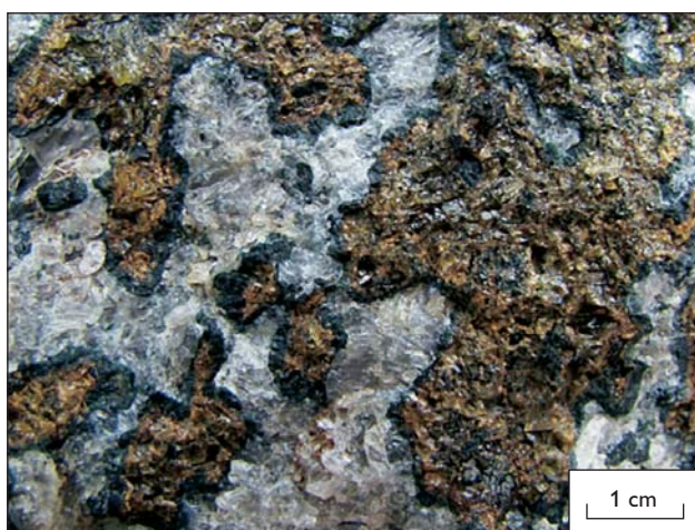
Fig. 3. Spinel-bearing plagioclase lherzolite showing the breakdown of olivine and plagioclase to form coronas of clinopyroxene and orthopyroxene. The stability limits of the plagioclase lherzolite are below c. 9 kbar and 1200°C, and the reaction would have occurred between about 700°C, 4 kbar and 870°C, 7 kbar. Location at 63.932°N, 51.219°W.
