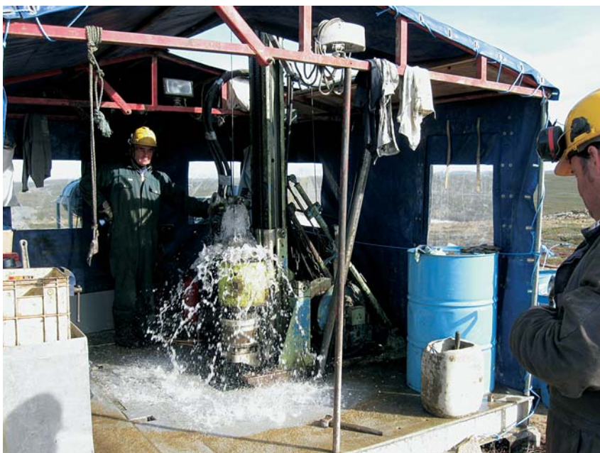
Fig 3. Drilling operations near Blokelv in Jameson Land. Three-metre-long cores are drilled at a time, and each time a core is retrieved water is pouring out of the drill hole.
