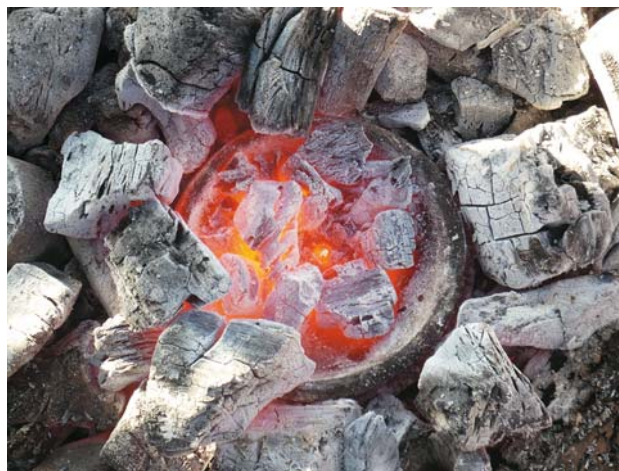
Fig. 3. Molten gold in the centre of the glowing clay bowl and charcoal.
