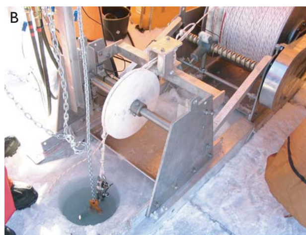
Fig. 2. A: Lightweight gravity coring equipment (constructed by J. Boserup, GEUS) used during the drift of the GreenICE camp. B: Sediment cores were retrieved through a hole drilled in the ice.
