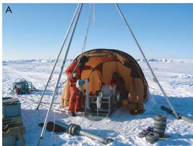
Fig. 2. A: Lightweight gravity coring equipment (constructed by J. Boserup, GEUS) used during the drift of the GreenICE camp. B: Sediment cores were retrieved through a hole drilled in the ice.
