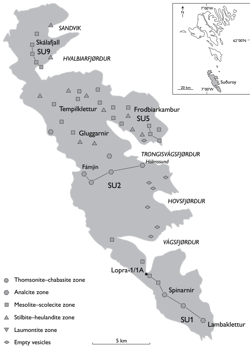
Fig. 5. Distribution of zeolite zones on Suðuroy and on sections SU1, SU2, SU5, SU9 and in the Lopra-1/1A borehole.
