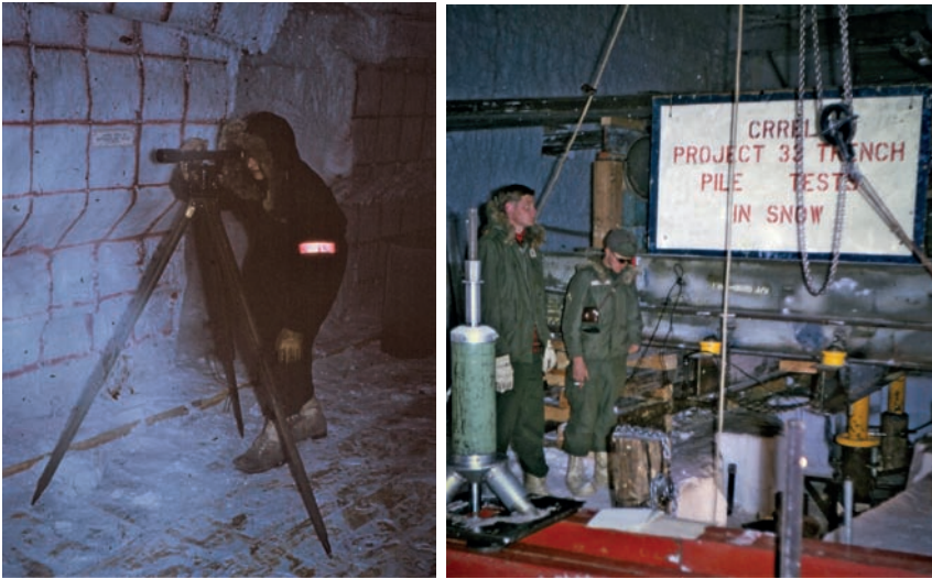
Fig. 2. USACE-applied glaciology research at Camp Century. Left: Measuring the deformation of firn in 1961. Right: Measuring the compressive strength of firn in 1964. Photos: Søren Gregersen.
