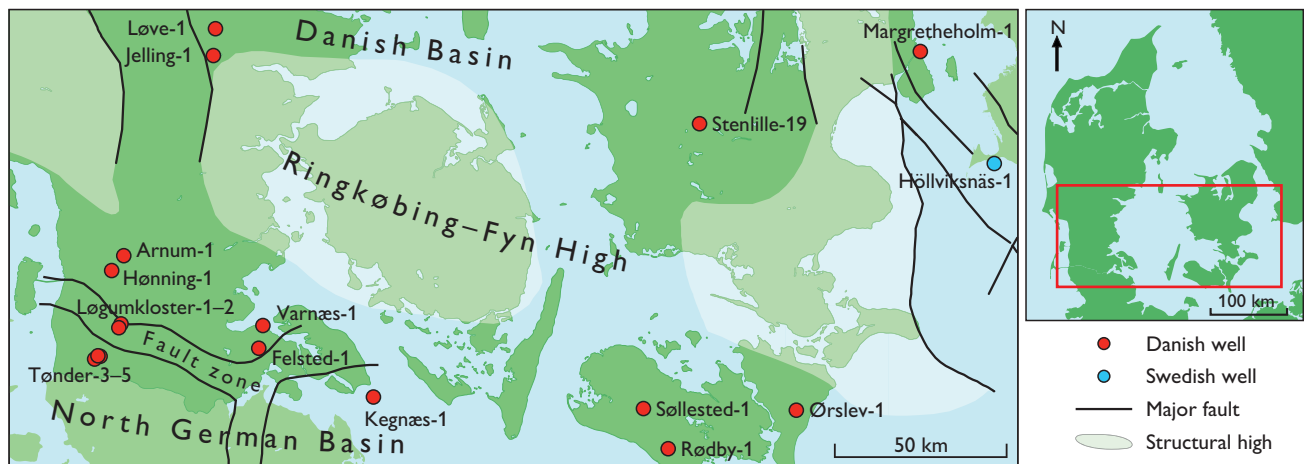
Fig. 1. The approximate extent of the Bunter Sandstone Formation in southern Denmark and adjacent areas (as delimited by the map frame), showing major structural elements and locations of investigated wells. Maps showing e.g. the extent, thickness and data sources of the Bunter Sandstone Formation are available from the WebGIS portal at the Geological Survey of Denmark and Greenland ( http://dybgeotermi.geus.dk/ ).
