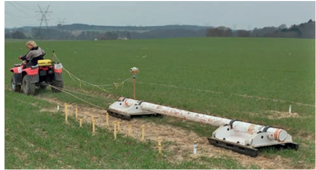
Fig. 3. The EMI survey system towed behind a vehicle. The c. 4 m long sensor is located inside a white tube on two sleds. The GPS sensor is mounted in the front of the tube above the transmitter coil. A data logger and a computer controlling the data acquisition are placed on the vehicle.
