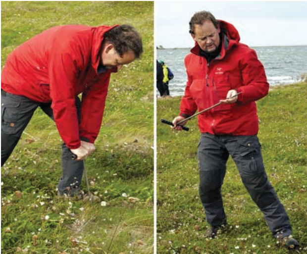
Fig. 2. Traditional geological mapping using the spear auger.
