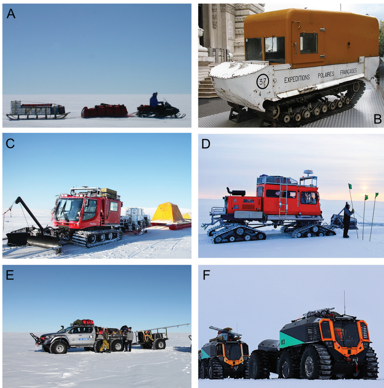
Fig. 13 Photographs highlighting the light traverse vehicles itemised in Table 2. A: Snowmobile. Photo: William Colgan. B: Weasel. Photo: Wikimedia Commons. C: Pisten Bully. Photo: Patrick Smith. D: Tucker SnoCat. Photo: Patrick Smith. E: Arctic Truck. Photo: Patrick Smith. F: Sherp. Photo: Henrik P.Ø. Lassen.
