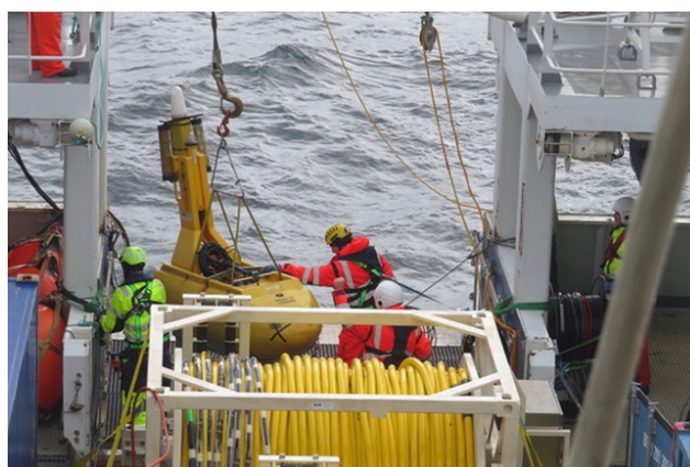
Fig. 10 Photographs from the Jammerbugt seismic acquisition. (a) The Faroese research vessel Jákup Sverri about to leave Hirtshals harbour (northern Jylland) for the seismic acquisition. (b) Deployment of the streamer tail buoy. In the foreground, one of the two winches with the solid-state streamer cable (Sercel Sentinel SSRD; yellow cable). Photographs: Thomas Funck.
