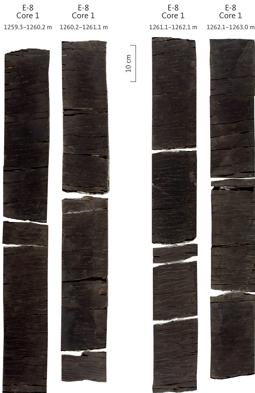
Fig. 29 Slabbed core section of the Hodde Formation from the E-8 well (Fig. 28). Note that the formation is totally bioturbated.
