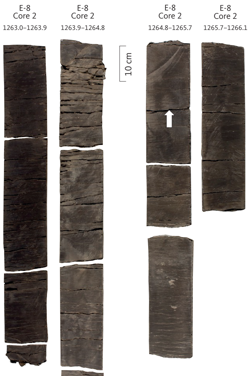
Fig. 24 Slabbed core section of the Nora and Hodde Formations from the E-8 well (depth intervals in metres). Note that the Nora Formation is muddy at this location, as indicated by the brown colour of the rock, and the upper boundary is therefore not distinct in the core but is placed at a distinct change in gamma-log readings ( white arrow ). The overlying Hodde Formation consists of bioturbated, dark brown to blackish mud in this part of the North Sea.
