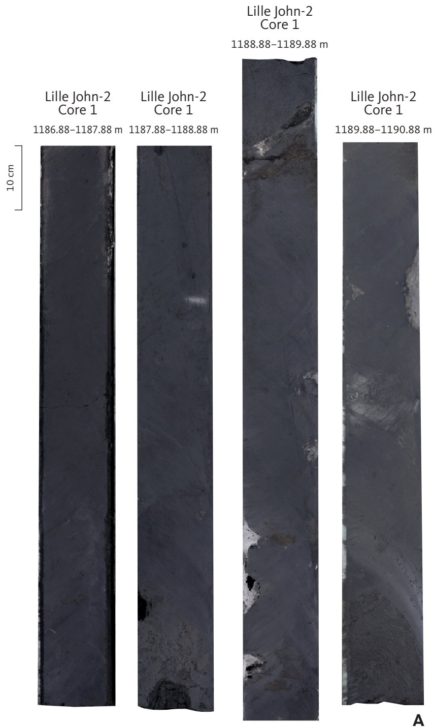
Fig. 43 Core image of the lower part of the Vagn Formation in the Lille John-2 well. Slabbed core under normal light ( A ) and UV light ( B ). Note the sharp boundary (arrow) between the Miocene Gram Formation and the Pliocene Vagn Formation on the UV processed image; the boundary between the Gram Formation and the underlying Lula Formation (Lille John Member) is at 1188.15 m. The full extent of the cored section is shown in Fig. 36B.
