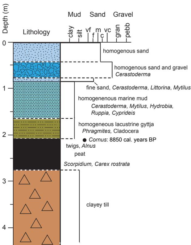
**Fig. 2** Sedimentological log of vibrocore 502017-1, collected at 56.033°N, 10.326°E, at a water depth of 9.1 m. The presence of peat with remains of *Alnus* overlain by lacustrine gyttja and marine mud shows that the area has been transgressed by the sea. A fruit stone of *Cornus sanguinea* was dated to c. 8850 cal. years BP (Table 1).
