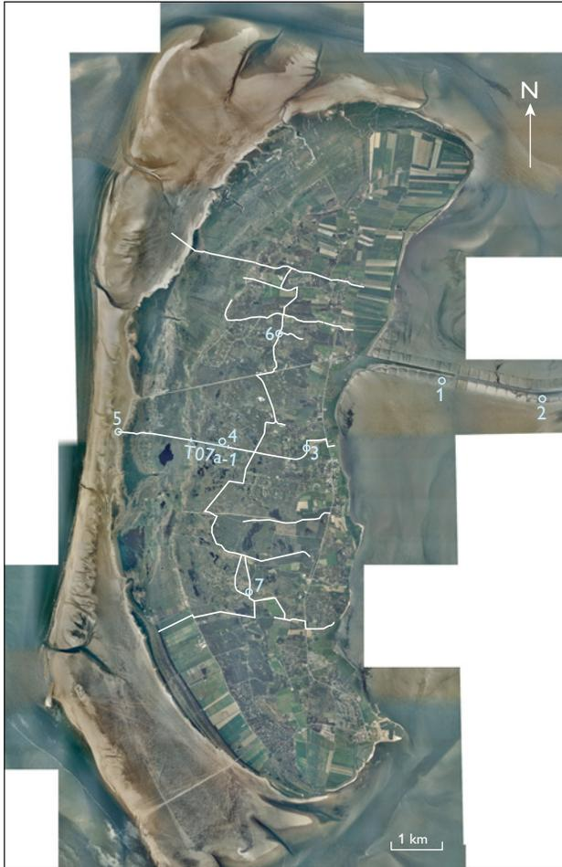
Fig. 2. Orthophoto of the Rømø barrier island. The location of GPR reflection profiles and the seven core wells are shown. Very wide tidal sand flat characterise the north-western and south-western parts of Rømø. Rømø island is dominated by aeolian dunes that are migrating eastwards. Copyright Scankort.
