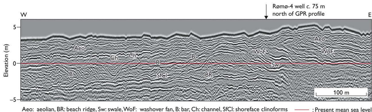
Fig. 5. West-east-trending ground penetrating radar profile T07a-1 from Rømø. The upper part of the section consists of aeolian sand. For location see Fig. 2.
