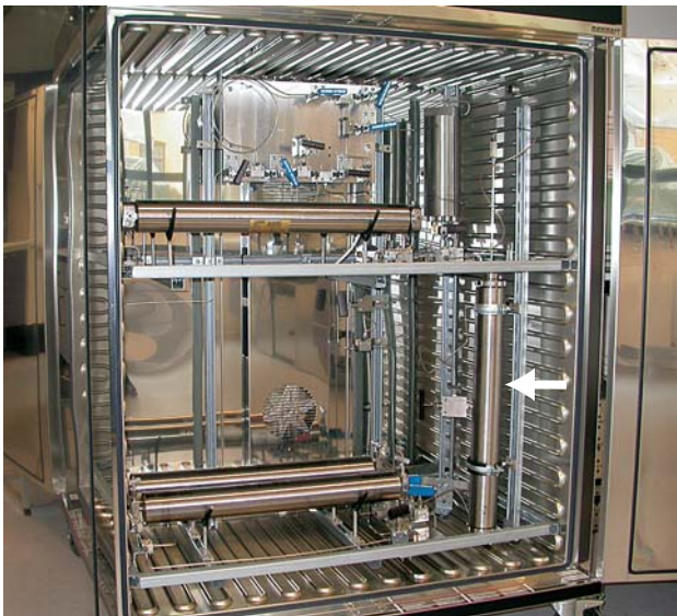
Fig. 1. Oven with high-pressure equipment used for the experiment described in this paper. The oven is 160 cm high. The arrow shows the core holder that was used for the experiment.
