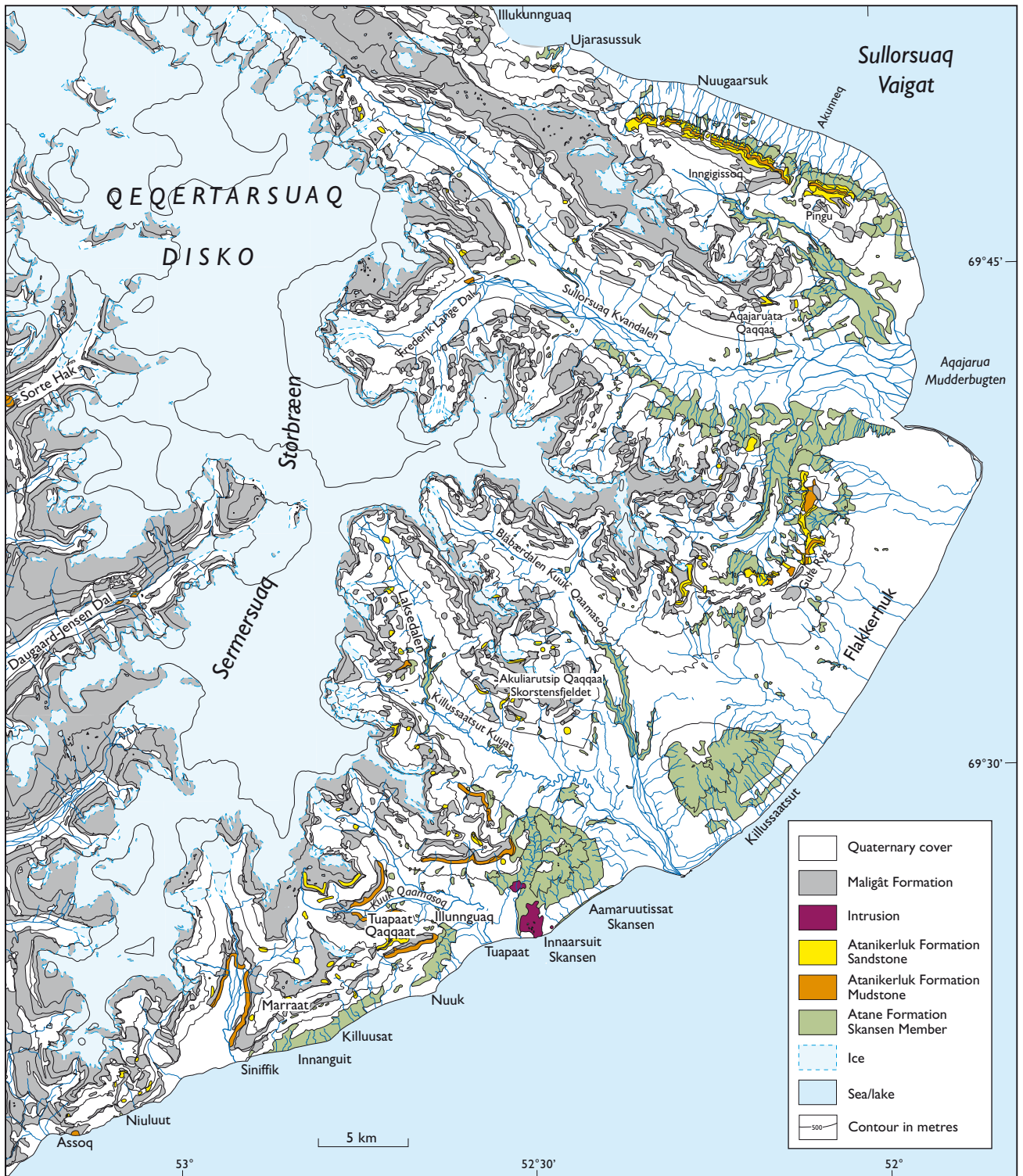
Fig. 124. Geological map showing the distribution of the Atane and Atanikerluk Formations on eastern Disko, simplified from A.K. Pedersen et al. (2001). Note that the outcrops of the Atanikerluk Formation are discontinuous. Contour interval is 200 m. For location, see Fig. 2.
