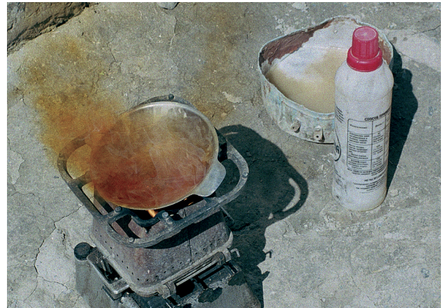
Fig. 5. Acid treatment. Boiling the gold concentrate with concentrated nitric acid. The process releases very toxic brown fumes of nitrogen oxides.
