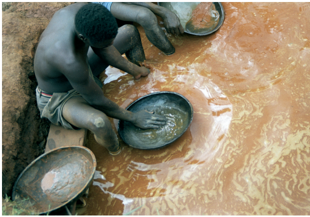
Fig. 2. Amalgamation in Tanzania. Note the shiny spots of metallic mercury in the pan.
