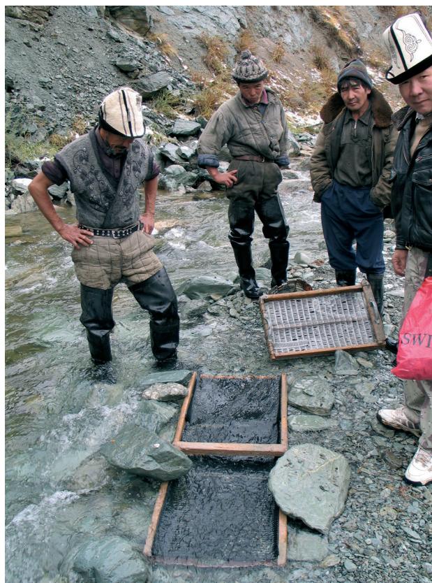
Fig. 1. Sluice for recovering placer gold in a stream in Kyrgyzstan.
