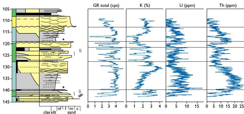
Fig. 3. Spectral gamma logs from 40 m of the core from borehole 247801. Note the difficulty in interpreting the total gamma radiation log, the negative correlation between K and Th content, and the absence of maxima on the U log. The core section is located in Fig. 2. Yellow: sandstone, grey: mudstone, black: coal or plant debris, black stars: pyrite. cps: counts per second. The total gamma radiation (GR) may be compared to the radiation measured in the borehole (Fig. 2).
