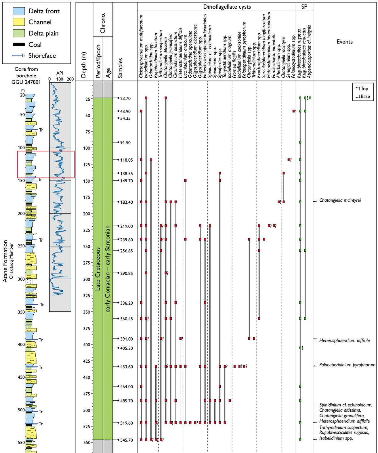
Fig. 2. Data from borehole 247801: a simplified sedimentological log of the entire core (566 m), a gamma log measured in the borehole to a depth of 320 m, and the new range chart for the dinoflagellate cysts in core samples. **API**: American Petroleum Institute units. GGU 247801 is located at 70°19.87'N, 52°55.8'W. The framed interval is shown in Fig. 3. The drill site is shown in Fig. 1B.
