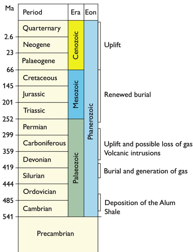
Fig. 2. Timing of main events affecting the gas potential in the Alum Shale in southern Scandinavia.
