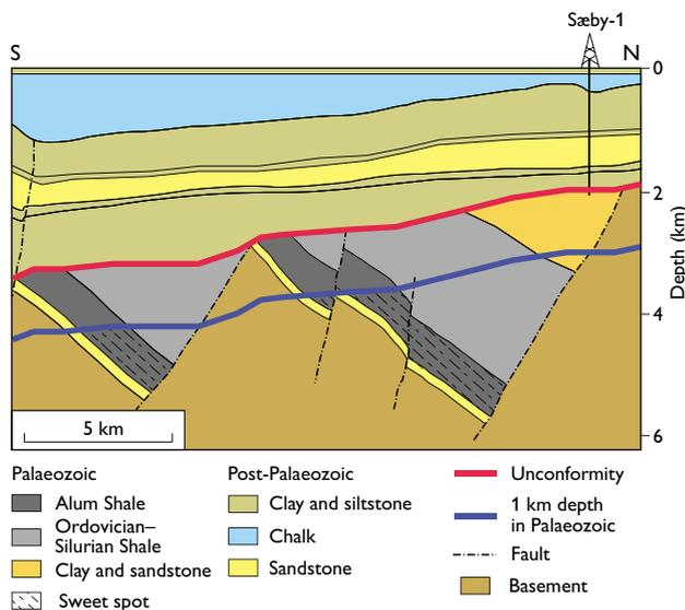
Fig. 4. Conceptual cross section showing the subsurface geology in northern Jylland. The Alum Shale is present in tilted fault blocks below the Caledonian unconformity. Sweet spots are the areas with lowest risk of gas leakage during Late Palaeozoic uplift and are defined as regions where the Alum Shale is overlain by more than 1 km of Lower Palaeozoic strata. Modified and generalised from Mogensen & Korstgård (2003).
