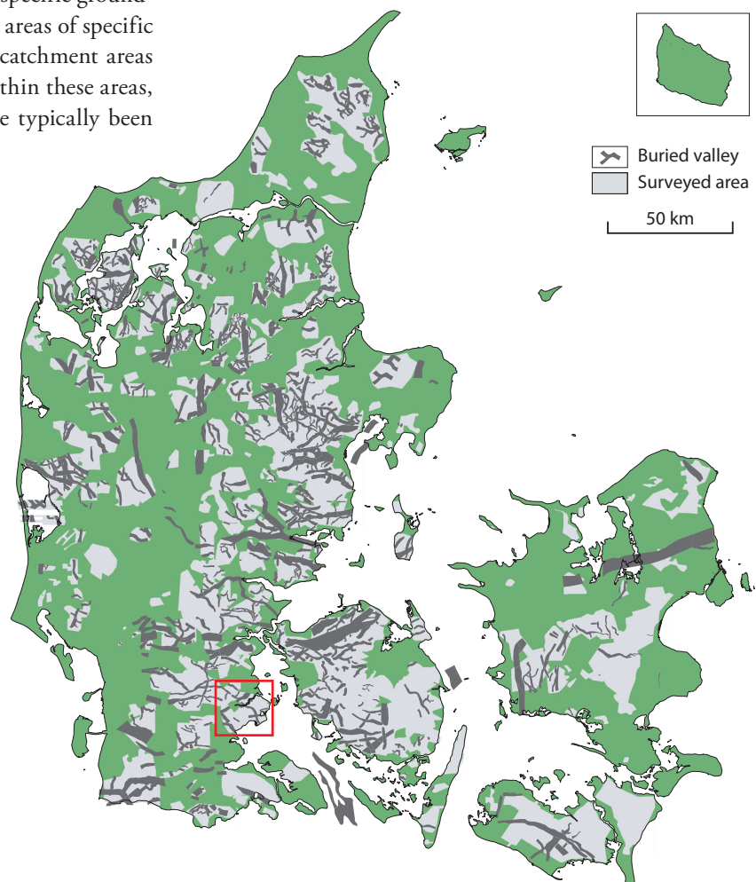
Fig. 1. Mapped buried valleys in Denmark as of end 2015. The mapped valleys are shown as dark grey polygons and the TEM-surveyed areas are shown in light grey. The Haderslev area covered by Fig. 2 is highlighted with a red rectangle.
