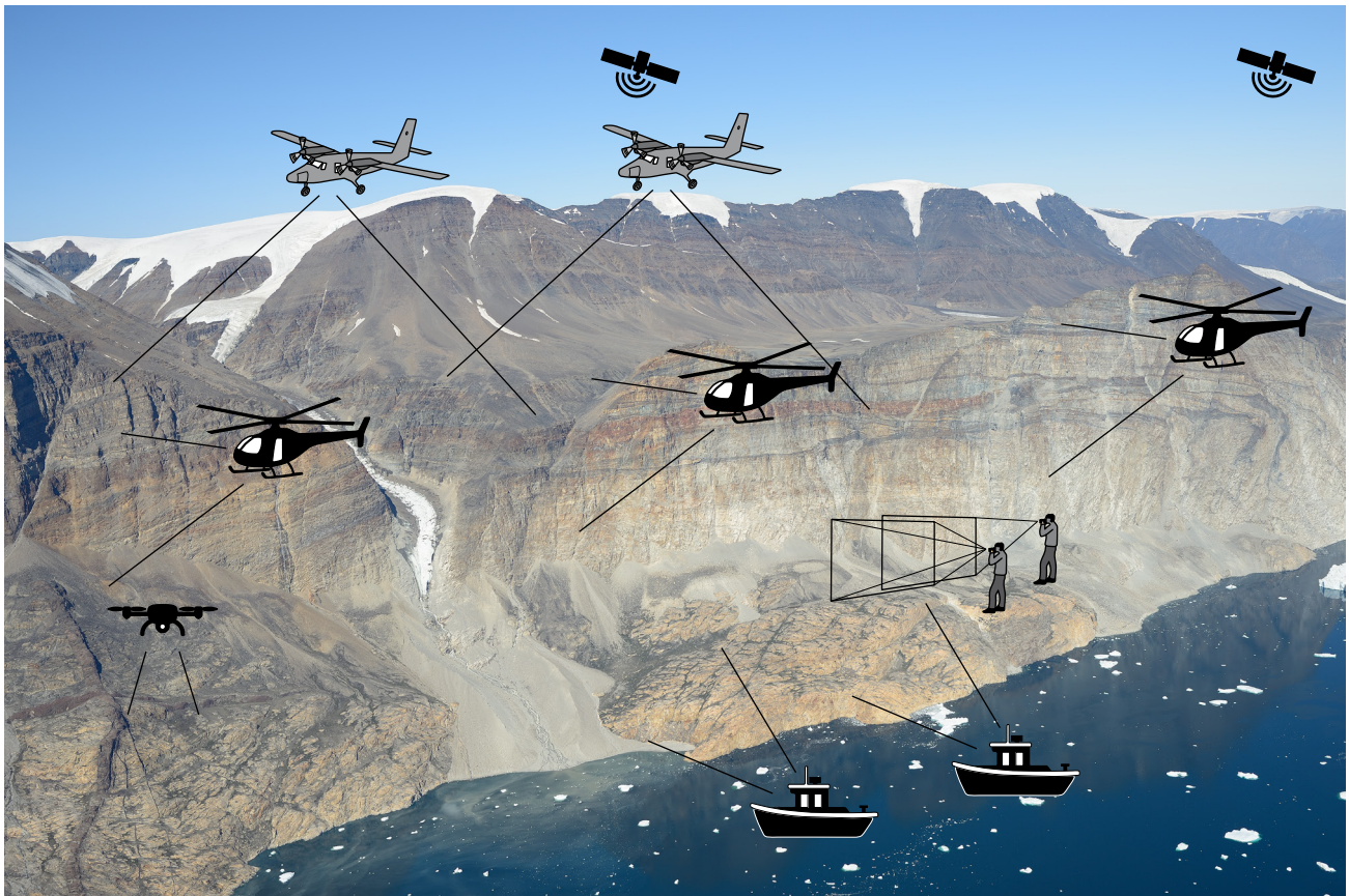
Fig. 1. During field work new stereo imagery is normally collected from helicopters or boats, but could also be collected from smaller fixed-wing aircraft, drones or while walking.
