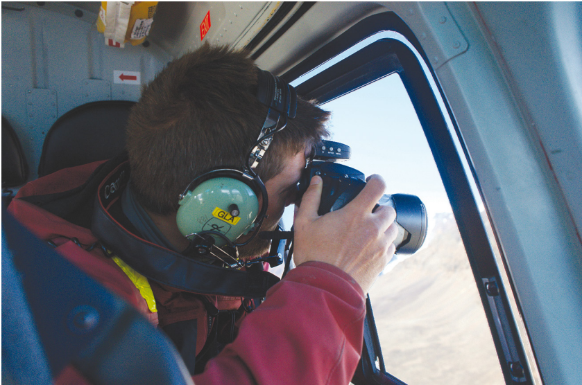
Fig. 4. Stereo images collected from helicopter using a hand-held digital camera. This method makes the data acquisition very mobile and fast. The location of the camera is registered with Global Navigation Satellite Systems. Photo: Jonas Petersen.
