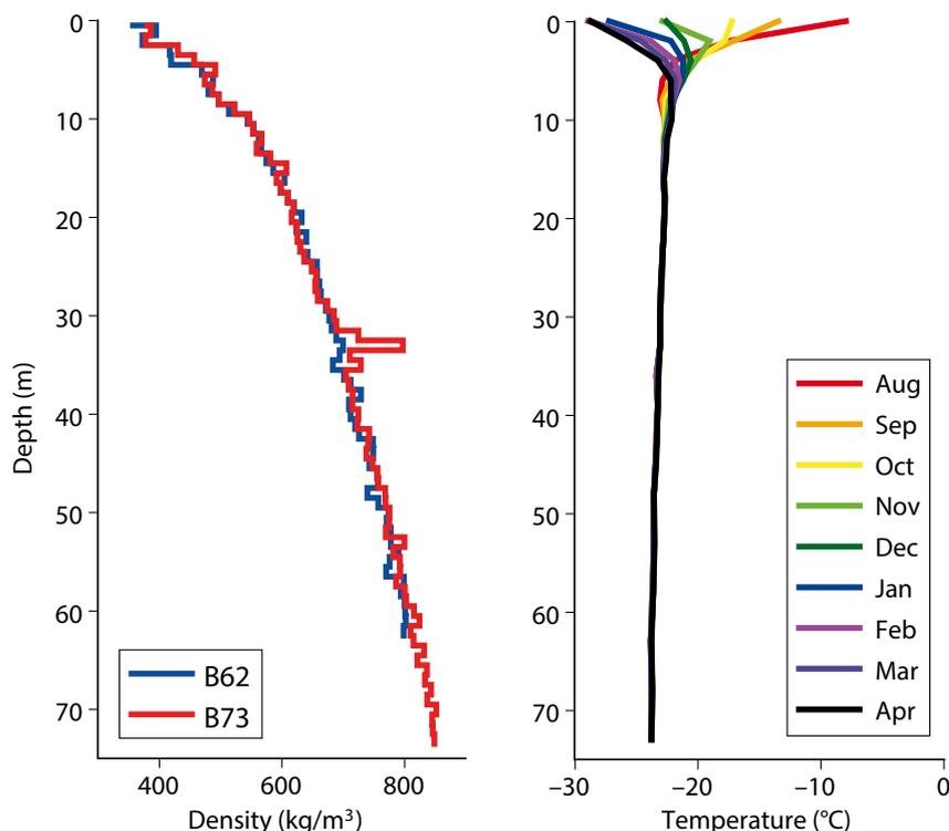
Fig. 4. **Left:** Near-surface firn density profiles measured both inside (B73) and outside (B62) the debris field. The high-density layer between 32 and 35 m depth within the debris field likely reflects enhanced compaction during the *c.* 1960–1964 active period. **Right:** Near-surface snow/ice temperatures at B73 inside the debris field. The annual temperature cycle penetrates to *c.* 12 m depth, with year-round firn temperatures remaining *c.* -24°C below this depth.
