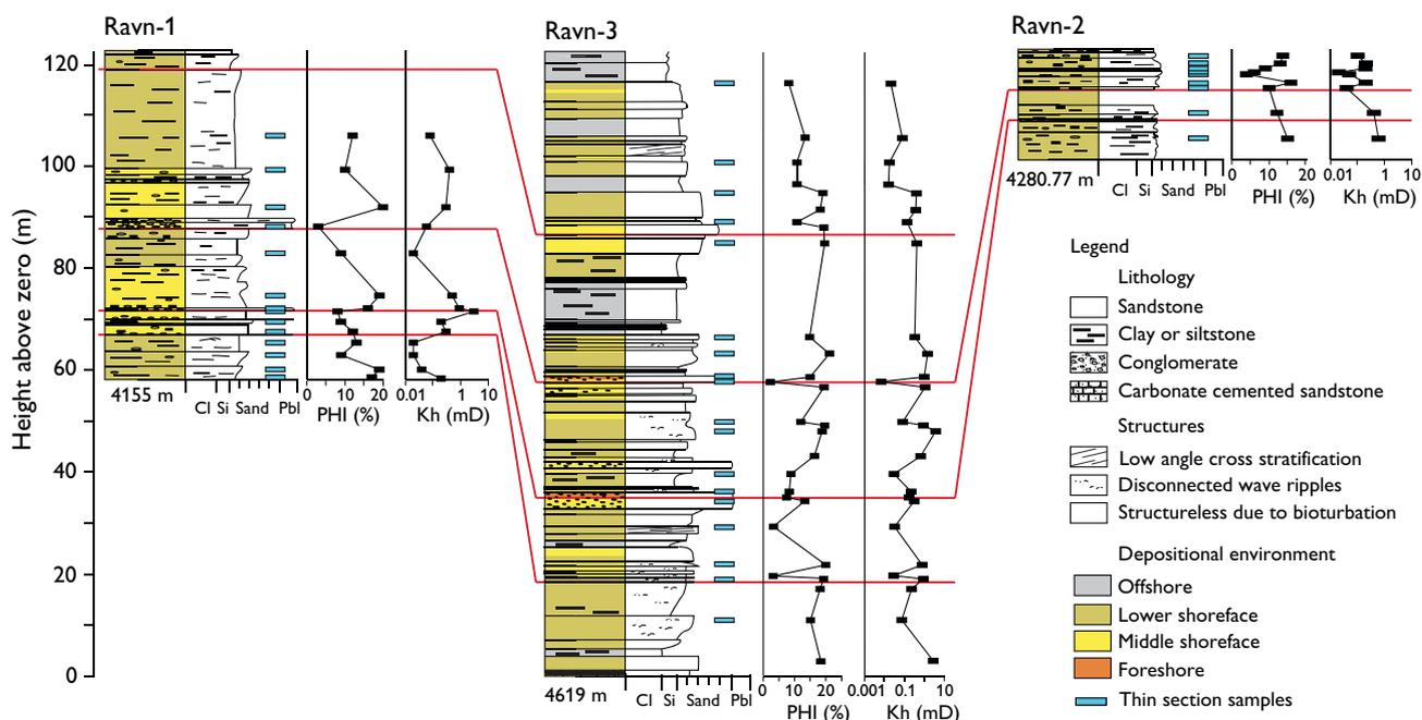
Fig. 2. Correlation panel of the cored parts of the Ravn-1, -2, and -3 wells. The Ravn-1 and Ravn-2 logs are modified from Johannessen (2010), whereas the Ravn-3 core was logged for this study. The depositional environment described in the Ravn-3 well (Panterra 2011) is based on ichnofacies. **PHI**: Porosity. **Kh**: horizontal permeability. **Cl**: clay. **Si**: silt. **Pbl**: pebble.
